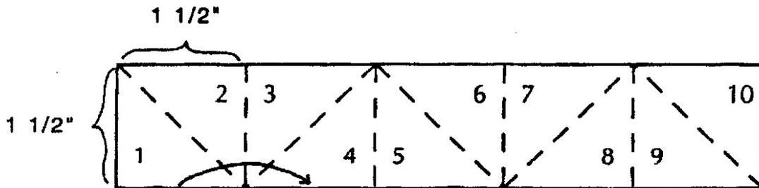
Use an exacto knife to score along each vertical and diagonal line with the exception of the vertical line on the right side. Score each line approximately half way through the thickness of the card. Do not cut through.
