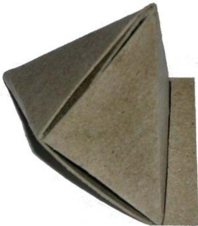
There will be a small amount of cardboard extends from the edge of the triangle form. Mark the excess and remove it so that it is flush with the side of the form. This excess will allow for variances in the thickness of the cardboard used for the form.
